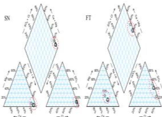
Figure 4. Location of water samples in FT and SN samples in the Piper Diagram
