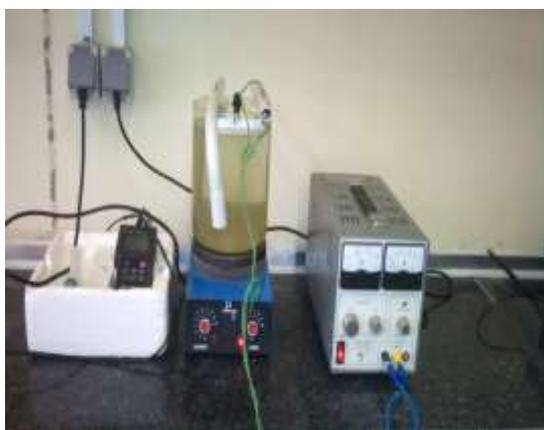
**Figure 2. Pilot Used in Electrocoagulation Process**
